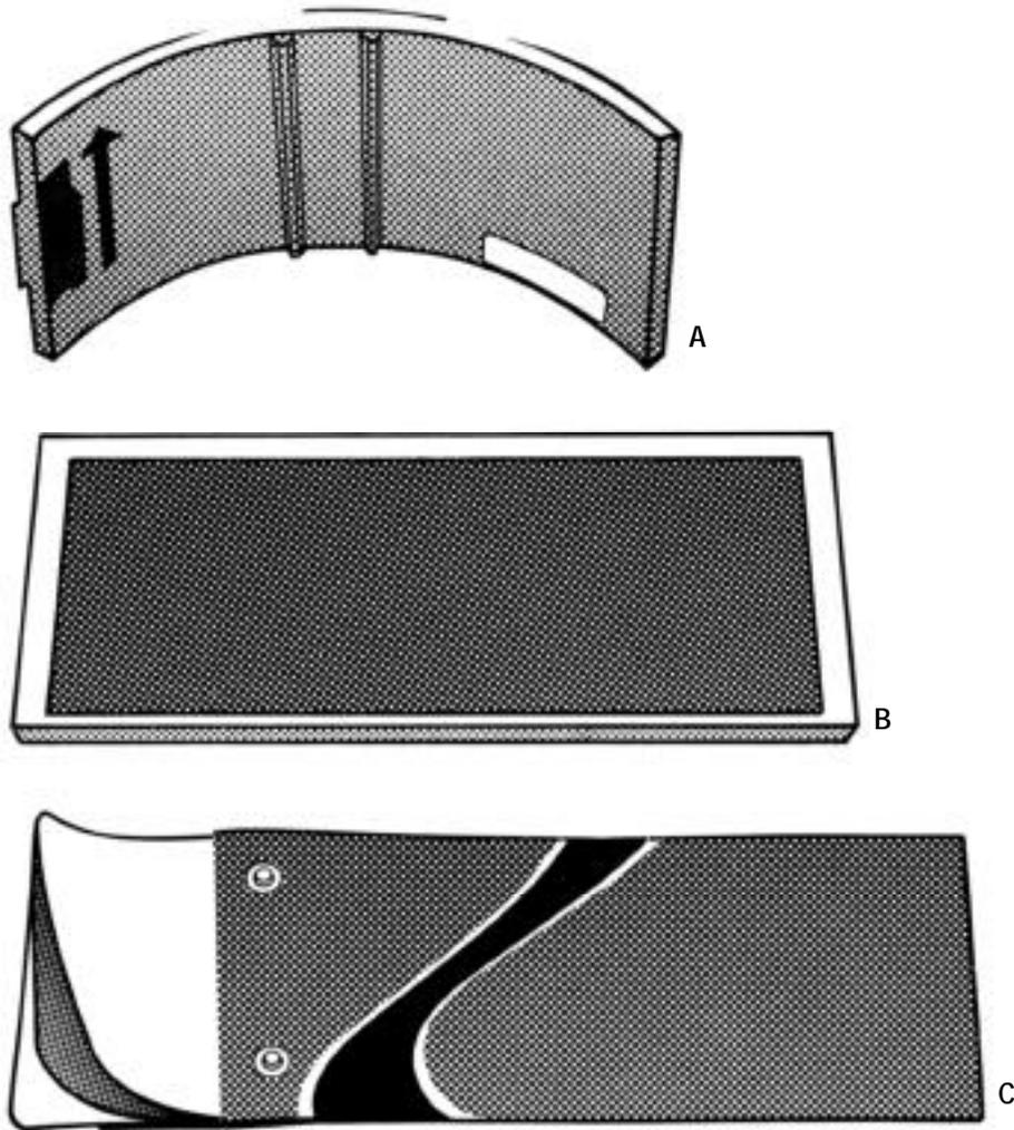
**Illustration No. 4:** Film cassettes. Figures "A" and "B" are rigid cassettes. In a rigid cassette, the intensifying screens are attached to the inside cover and base of the cassette. When the panoramic film is placed in the cassette, it lies in-between the screens. Figure "C" is a flexible cassette which has an opening at one end creating a pouch. The panoramic film is placed between two removable, flexible intensifying screens which are then slid into the pouch.
